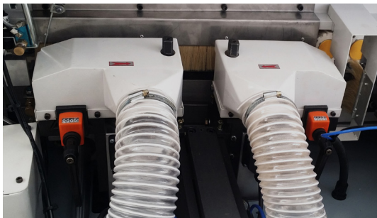
Pre-milling unit: 2x2.5 HP high speed motors, stable and accurate, ensures a perfect milling of panel edge.
