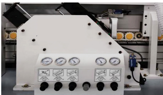
End trimming unit. Two motors are sliding on two linear guides
