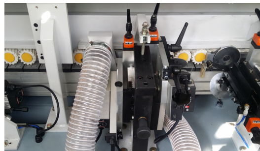
Pre-milling unit: 2x2.5 HP high speed motors, stable and accurate, ensures a perfect milling of panel edge.
